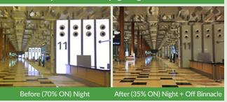
Dimming of lights in T3 Departure Hall during low-use periods at night and switching off nonessential Binnacle lighting
