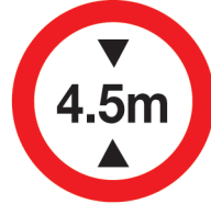
Height limit (Vehicle of height 4.5m or vehicle carrying load exceeding height of 4.5m is not allowed to enter)
