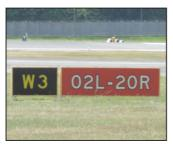
White-on-red mandatory signs are located at runway holding positions (explained in a later section). These signs warn drivers and aircraft that the runway indicated on the sign is ahead: drivers shall exercise caution so as not to inadvertently enter the runway and cause
