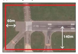
A defined area, including the runway and stopway if provided, that is intended to reduce the risk of damage to aircraft running off a runway, and to protect aircraft flying over the area during take-off or landing operations.
