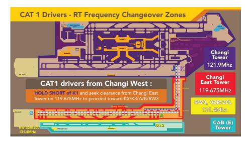
Drivers heading to Changi East via North Loop taxiways shall hold short of taxiway K1 and seek clearance from Changi East Tower on 119.675MHz. An example of the associated RT procedures is given in Section 5.
