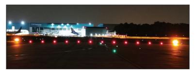
Runway holding positions are accompanied by steady red stopbar lights and alternating flashing amber runway guard lights.
