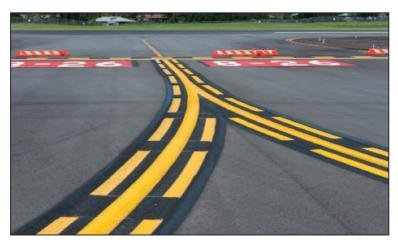
The Enhanced Runway Ahead Markings, also known as the Enhanced Taxiway Centreline, are additional dashed yellow lines on each side of the regular solid yellow taxiway centerline. The dashed yellow lines extend for about 50m from the runway holding position. The additional dashed lines provide additional visual indication that drivers are approaching a runway.
